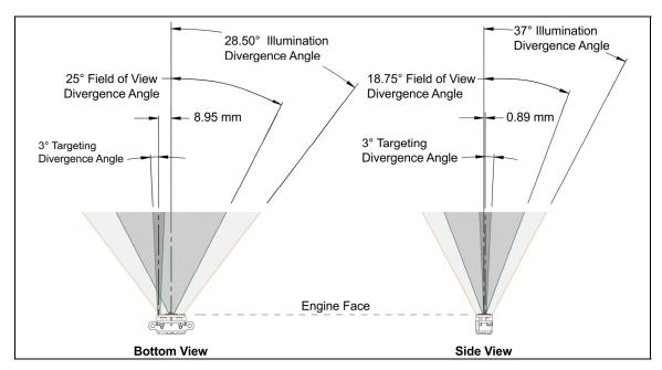
Figure 14. IS4910 Optical Clearance Specifications
